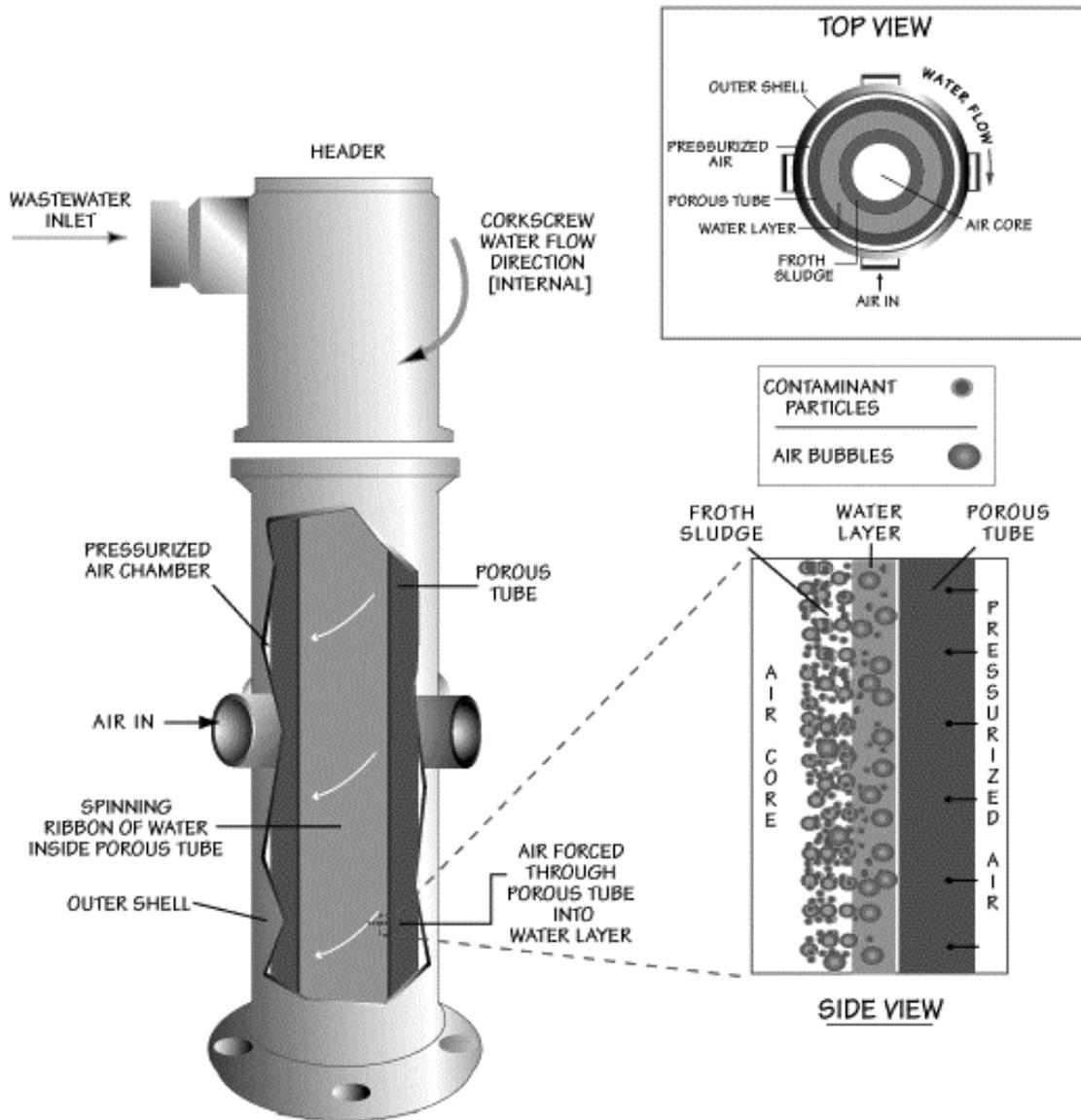
forced through the porous tube generates bubbles on the inside surface due to high shear. These bubbles are extremely buoyant in the centrifugal field because of the effective radial pressure gradient in the swirl layer generated by the hydrocyclone action. The bubbles accelerate toward the inner surface of the swirl layer. In addition to creating the radial acceleration of the bubbles, the centrifugal field also aids in the classification of particles with densities different
