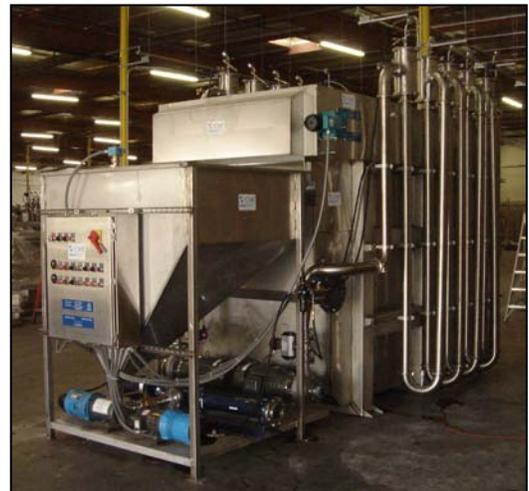
The equalization limitation also created a challenge in effectively treating load variances. A system that could adjust "Real Time" to follow TSS, FOG, and COD/BOD fluctuations was required. Since the LSGM technology is based on the "insitu" treatment principal, reaction times from chemical adjustments occur within seconds rather than minutes or hours. This enables the Client to effectively maximize reduction rates allowing the GEM System to accommodate inadequate equalization scenarios.
